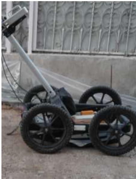
*Figure 5: GPR equipment (Ground coupled system).*
